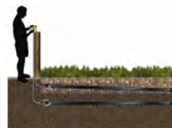
Figure 1: Example of 2 sensor installation in pasture with bottom sensor used to access root zone and canopy.
